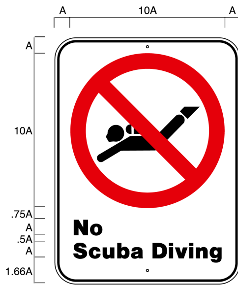
Grid Format C: Two-line legend with the word "No" alone on the first line. The first legend line is closer to the circle than in Grid Format B, to compensate for the empty space after the word "No".
