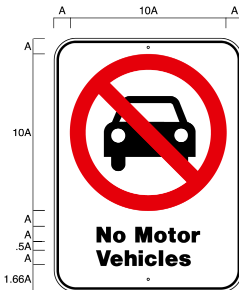
Grid Format B: Two-line legend. The two lines are aligned flush left, and then the longer line is centered on the panel.
