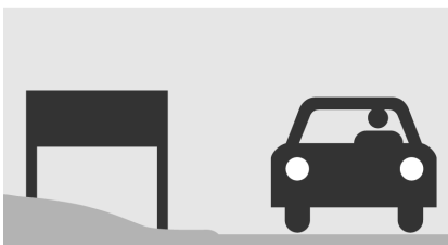
Post lengths adjusted for a grade sloping up from the road
